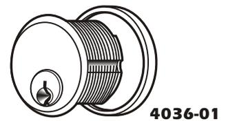
Standard diameter five-pin unit with MS® cam, suitable for use with Entry Trim. All brass construction with front "scalp" available in finishes 628, 313 and 335. Available in quantity all keyed different (KD), in pairs (KA2) or fifty alike (KA50). Any other make standard Mortise cylinder with MS® cam can be used to "key in" with existing systems.
