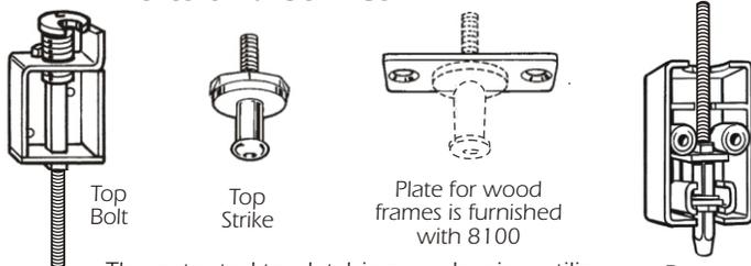
The patented top latching mechanism utilizes a rotating Top Bolt which deadlatches around the Header Strike, interlocking the door to the frame. For wood frames, an additional plate is supplied for securing the Header Strike. The hexagonal, hardened steel Bottom Bolt is shielded in a cast housing for strength and stability.
