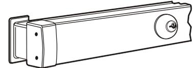
For management control of dogging. Any standard 15/16" to 1-1/8" long Mortise cylinder with MS® cam can be used in a pushbar prepared at factory with Cylinder Dogging kit. Cannot be used with Alarm, EL or LR options.
