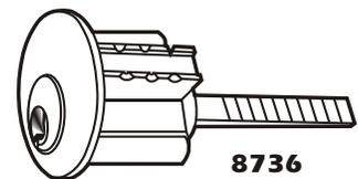
Standard five-pin unit with spindle to suit Surface Vertical Rod exit devices. All brass with same choices of keying as Mortise cylinder. Available in finishes 628, 313 or 335. Any other make standard Rim cylinder can be used to key in with existing systems. Note that if entry trim is specified for cylinder use, the cylinder must be Mortise type, regardless of exit device.
