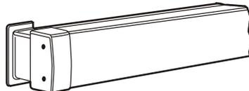
Dummy pushbar with no latch mechanism but with either a single or dual monitor/signal switch. Most common application is in conjunction with a maglock where bar is used to turn off magnet and allow exit from building. Dual switch version allows redundancy where required by code or the operation of a signal device along with maglock. Specify door type and width when ordering. Available in all exit device finishes.
