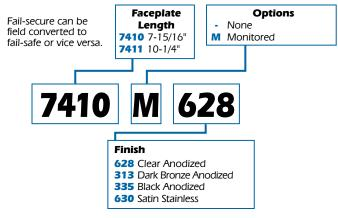
\*Modular Packing Program - match body kit with faceplate kit to complete. Use 7400A for standard jambs and 7401A for radius stile mounting. No finish designation required.
