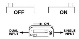
Two operating modes are available. Set the mode with switch 1 on dip switch SW1.
