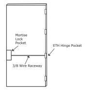
**Step 2** - Run the wires from the ETH hinge through the 3/8 race way starting at the ETH hinge & exiting into the mortise pocket.
