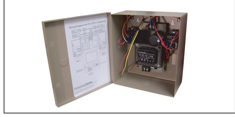
The PS1 and the PS1-2 are a heavy-duty low cost solution for powering electrically latch-retracting exit devices. The PS1 offers a single heavy duty 20 amp relay while the PS1-2 includes a pair of these 20 amp relays. These power supplies offer raw, unregulated DC current which is ideal for the extreme inrush requirement of most solenoid-driven electric latch-retracting exit devices. The power supply is housed in a sturdy yet compact metal enclosure.
