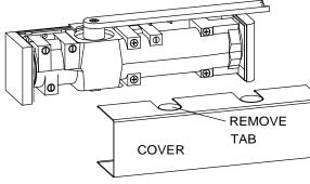
Remove tab that aligns with arm hub. Slide cover onto plate.
