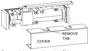
Remove tab that aligns with arm hub. Slide cover onto plate.
