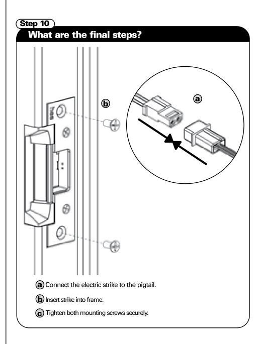
If binding between the latchbolt and keeper occurs you may need to horizontally adjust the electric strike.
