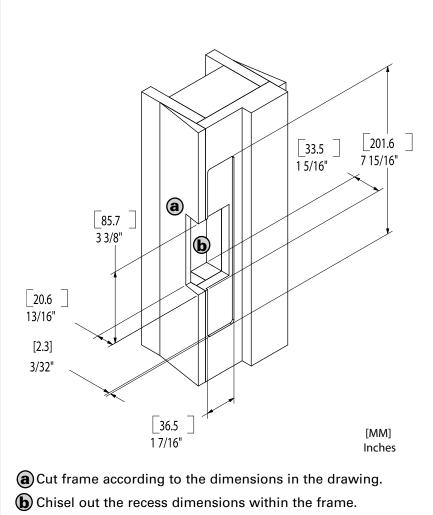
**•** For wood applications pre-drill pilot hole for mounting points with a #11 drill bit.
