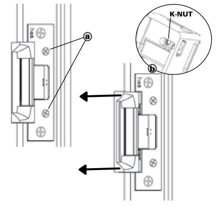
(a) Slowly turn the horizontal adjustment screws to adjust the strike in-frame. Do not remove the screws or completely rotate them more than 3 full turns.
