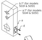
**B-2** Remove the two connecting screws (a) from the cylindrical drive unit (b). Rotate cylindrical drive unit 180 degrees. Reposition spacer (c) as found before disassembly. Remount drive unit with the two connecting screws.
