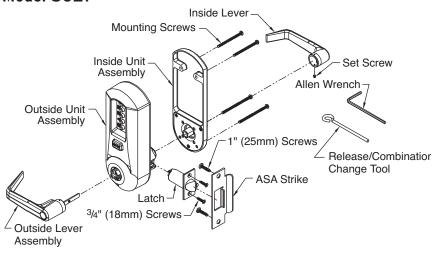
The Simplex 5000 (Model 5021 shown above) is a non-handed lock that is preassembled for left-hand installations. It is field reversible.
