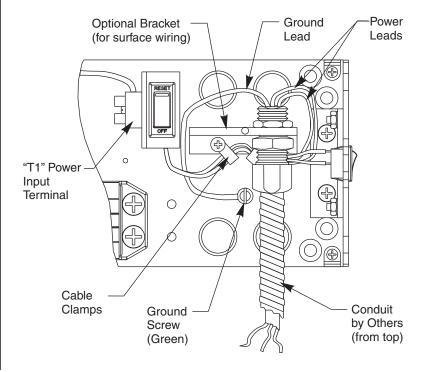
Ground Wire Connection – Ground wire must be secured to backplate under head of (green) ground screw nearest to "T1" Power Input Terminal. Screw labeled "GND".
