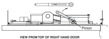
Step 8: Insert arm stud into slide block in track assembly. Secure by pushing in on the retainer clip that extends from the slide block in the track, until it is flush with the slide block (see illustration below).
