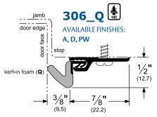
Minimum space between the door face and the stop is 3/16"; maximum space is 5/16".
