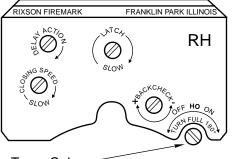
Do not use Backcheck as deadstop. This is an intensity valve not speed control.
