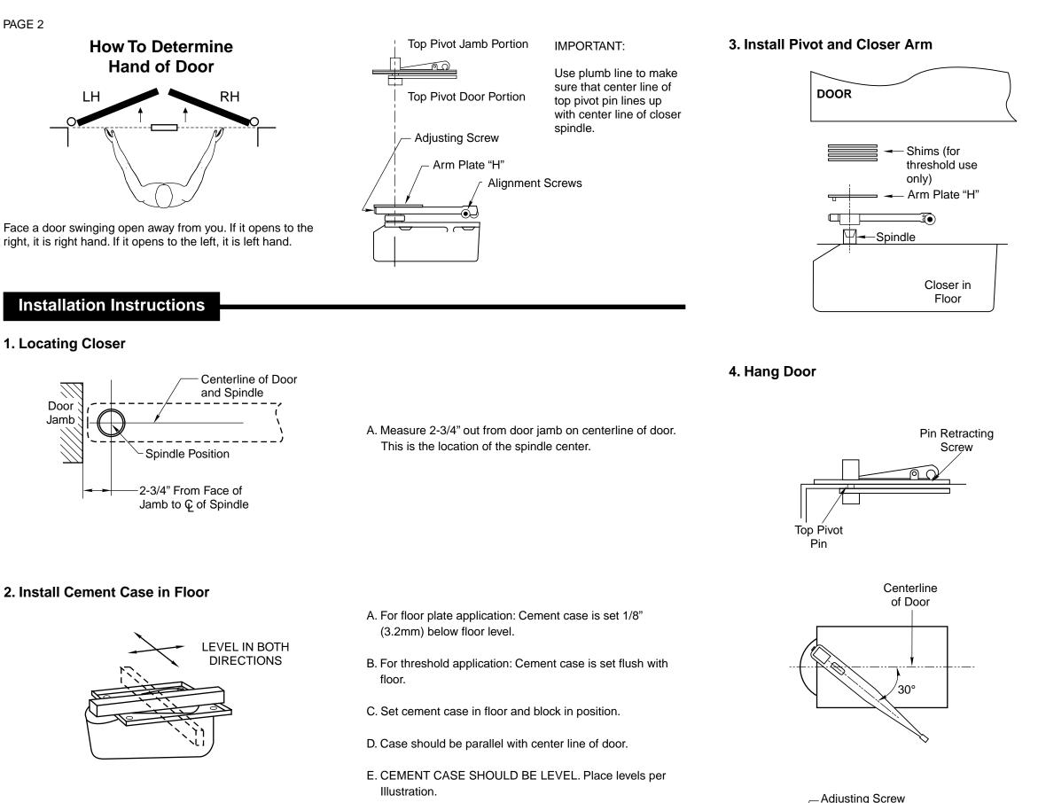
F. Grout in cement case with closer. Cement should not get between closer and case.
