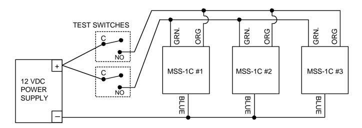
REMOTE TEST WIRING SHOWN WITH THREE MSS-1C SWITCHES. ANY NUMBER OF MSS SWITCHES CAN BE CONNECTED IN THIS WAY. NOTE THE TWO NORMALLY OPEN TEST SWITCHES. THEY SHOULD BE CLOSED ONE AT A TIME AND ALL MSS SWITCHES SHOULD GO INTO ALARM TWICE TO PASS THE TEST.
