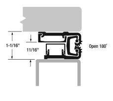
**MATERIAL:** Extruded 6063 T6 aluminum alloy with self-lubricating polyester thrust bearings.
