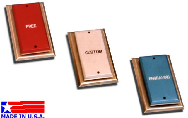
The **HIGHPOWER PUSHPLATE 100** series of heavy duty controls is designed for rugged applications. This series features a stainless steel back plate and anodized aluminum front plate that actuates a microswitch. Durability and Long Life are built in to this product since the travel of the front plate rather than the switch stop, limits the range of actuation. This insures maximum switch life and reliable service in the most demanding environments.
