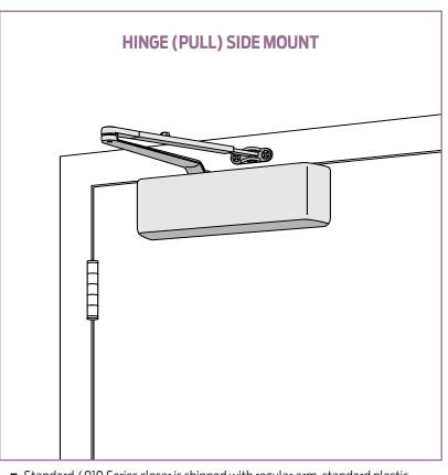
The 4010 is LCN's best performing heavy duty closer designed specifically for institutional and other rugged high traffic applications.
