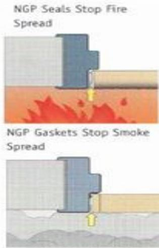
UL Test standards UL10C is Underwriter's Laboratories standard for testing of fire door assemblies to positive pressure with the neutral plane at 40" above the sill. This test standard is required to be met for all fire doors installed in jurisdictions that have adopted the International Building Code (IBC). The requirement for Smoke and Draft Control assemblies is also stated in IBC.
