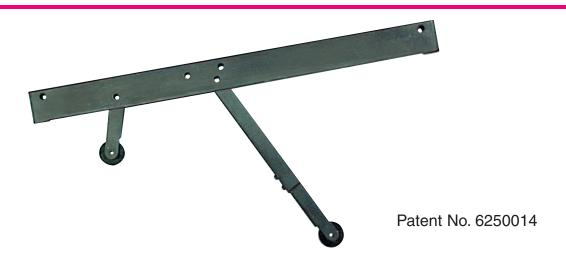
3780 Universal Coordinator is for pairs of doors up to 8' wide. The long arm holds the active door open until the short arm is depressed by the inactive door. When the doors are closed, the arms are hidden by the stop-mounted aluminum case.
