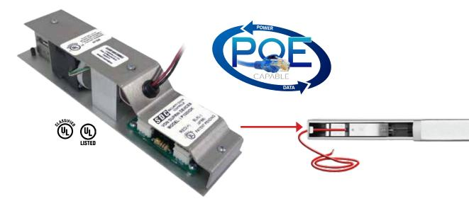
The SDC IP100 Series 12V PoE-Capable Electric Latch Retraction Kit enables electric access control and dogging of mechanical exit devices. When energized the motor retracts the exit device latch and pulls the pushpad\* into the dogged (depressed) position enabling momentary or sustained push and pull operation of the door.
