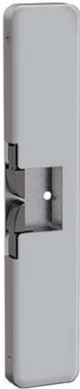
The 9400 series Genesis™ is a slim-line, surface mounted electric strike designed to accommodate rim exit devices with a 1/2" throw latchbolt. All components are completely encased within its 1/2" thick stainless steel housing, so no cutting on the frame is required for installation. Simply place the electric strike on the surface of the frame, align it with the exit latchbolt, and install.
