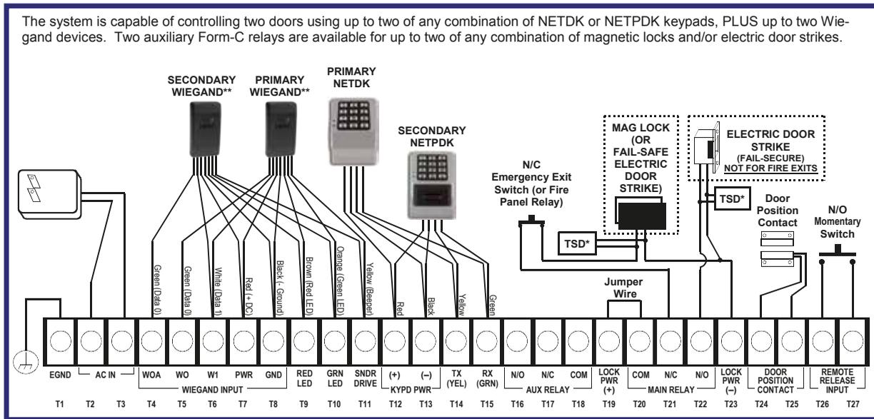
\*TSD = Transient Suppression Device (two supplied): Mount the TSD as close to the device to be protected as possible.
