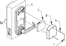
**Caution**: Over-tightening these screws could strip the threads in the housing or crack the cover.
