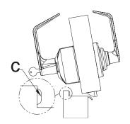
**Note:** Allow 24 hours for adhesive to set before testing. The door may be operated normally during this time.
