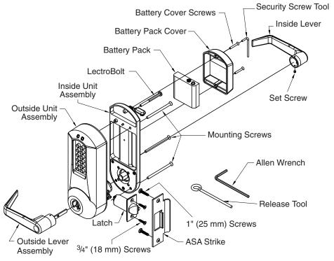
The E-Plex 5031 is a non-handed lock that is preassembled for left-hand installations. It is field reversible.
