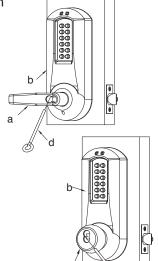
Insert the supplied tailpiece (e) vertically into the outside lever/knob (b) as shown. Make certain that you rotate the tailpiece so it will align with the interchangeable core. For screw cap type cylinders (Schlage) (g), the tailpiece must be assembled to the cylinder first with the tailpiece vertically as shown. Insert the core into the outside lever/knob.
