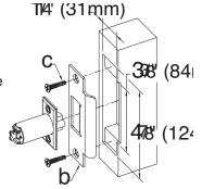
Caution: Check the operation of the latch by making sure that the deadlatch (a) stops against the strike (b) as shown and does not slide into the strike opening when the door is closed. If that situation occurs, then a total lockout may occur. This will void our warranty of the complete lock mechanism. If necessary, correct the door over-travel by using the rubber bumpers as described in Section N (Installing Rubber Bumpers).
