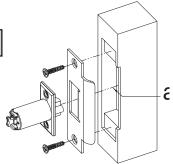
M-2 Mortise doorframe for strike <sup>3</sup>/<sub>32</sub>" (3 mm) deep minimum to dimensions shown. Secure strike (b) to the door frame using two 1" (25 mm) combination screws (c) (supplied).
