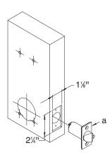
A-3 Secure the latch to the door using two <sup>3</sup>/<sub>4</sub>" (19 mm) combination screws (b) supplied. Latch unit faceplate must be flush with door (c).
