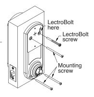
**Warning:** If using a power drill, please be careful not to over-tighten as this could cause damage to the mounting screws and threads.
