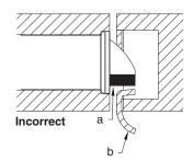
N-2 Mark locations where the gaps are approximately <sup>3</sup>/16" (5 mm). Make sure these locations are free from grease and dust. Peel the bumpers (c) (supplied) from their protective backing without touching the adhesive surface and stick them on the marked locations.
