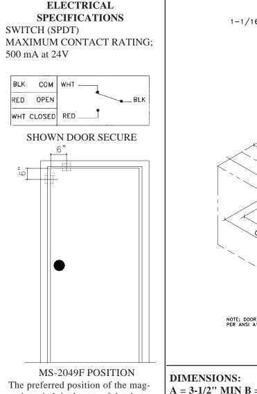
The preferred position of the magnetic switch is the top of the door, centered approximately 6" from the edge of the door, as shown. Contacts should be installed so that the door cannot be opened more than 2 inches without causing an alarm condition.
