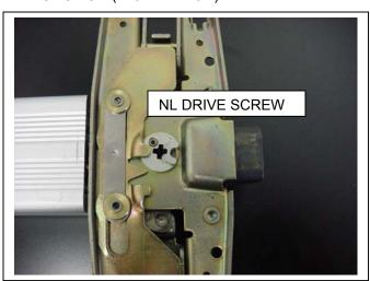
• SLIDE OUTSIDE CHANNEL FROM DEVICE AND INSTALL DOOR CABLE IN BOTTOM OF DEVICE BASEPLATE ASSEMBLY AS SHOWN BELOW.
