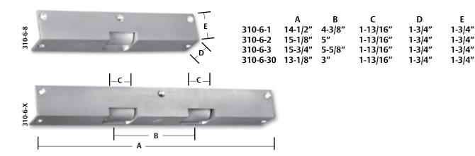
These industrial grade electric strikes are used on a pair of doors (without mullion) which are equipped with concealed, vertical-rod exit devices having a 1/2" or 5/8" throw latchbolt
