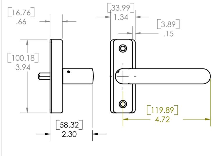
HUB MUST BE ON DIAMOND FOR PROPER INSTALLATION.
