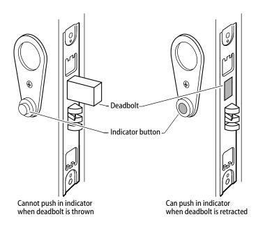
*Figure 3 — Testing the hotel indicator for proper operation*
