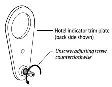
Figure 1 — Unscrewing the hotel indicator adjusting screw
