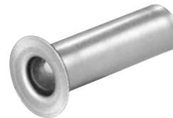
The BFB Bottom Fire Bolt eliminates the bottom automatic flush bolt and dust proof strike. The BFB is installed horizontally in the inactive door, with a mating hole in the edge of the active door. When subjected to 230°F the BFB projects a bolt, locking the leaves together.
