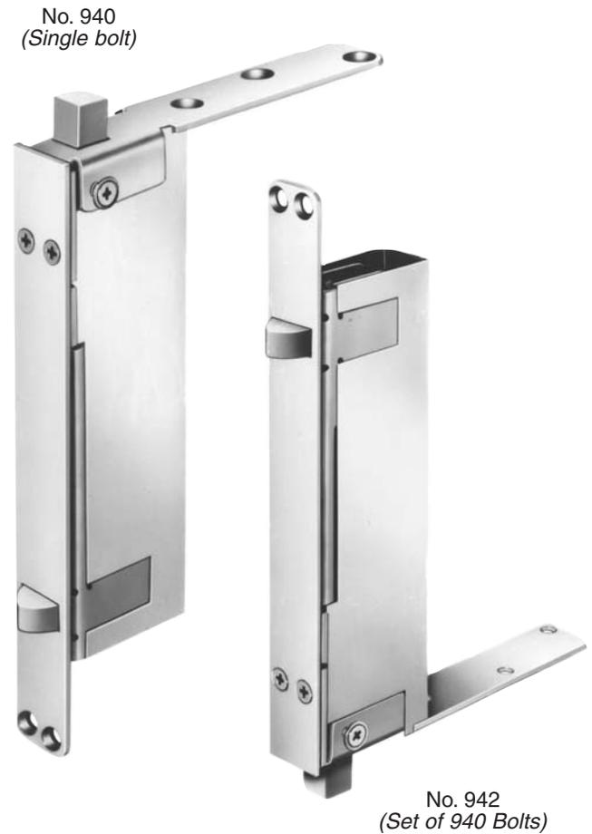
Automatic flush bolts are installed in the top and bottom of the inactive door. Closing the active door automatically extends both top and bottom bolts  $\frac{3}{4}$ " into frame and sill strikes, locking inactive door. Opening the active door retracts top and bottom bolts, releasing the inactive door. Manufactured and assembled in Dexter, Michigan.
