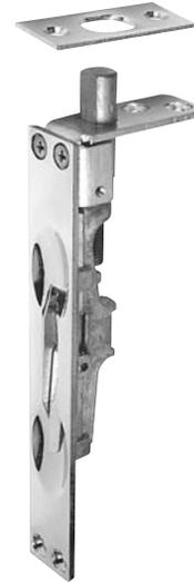
Manual Flush Bolt are installed in the inactive door. The lever mechanism extends the bolt head  $\frac{3}{4}$ " into the frame and sill strike, locking inactive door. All rods have  $\frac{1}{2}$ " adjustment for door and strike clearance.
