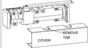
Remove tab that aligns with arm hub. Slide cover onto plate.
