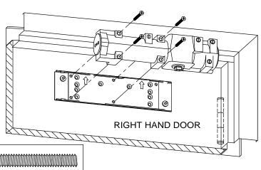
Place wrench on bottom pinion. Rotate pinion 5° TOWARD HINGE edge of door. With main arm parallel to door, place main arm onto top pinion. Fasten securely with pinion screw.
