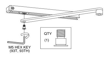
Adjust sweep, latch, backcheck and delayed action valves.
