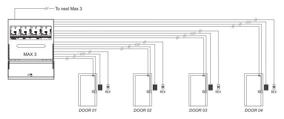
**Max 3** – The Max 3 cabinet configuration provides the simplest expansion of one to four doors per cabinet when the system needs to be installed in a central location.
