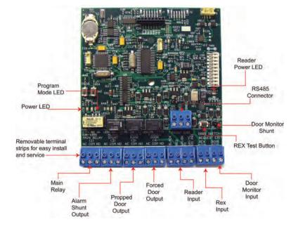
Max 3 Module - All transaction events are stored, and system programming decisions are made, in the Max 3 Module. Up to 64 door modules can be networked together per site with virtually unlimited sites.
