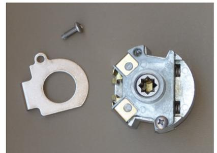
**Removing Cover From Retractor Mechanism**
