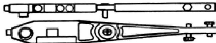
"S" TYPE ADJUSTABLE SIDE LOADING TOP ARM ASSEMBLY (1/2" Depth Top Rail)
