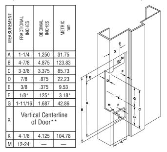
**7108, 7308** Aluminum & Wood Frames, 1-1/2" D **4108, 4308** Aluminum & Wood Frames, 1-1/2" D Any modular **A41, A43, A71** or **A73** with **B4708** faceplate
