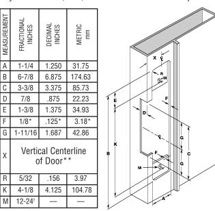
**7119, 7319** Steel & Wood Frames, 1-1/2" D **4119, 4319** Steel & Wood Frames, 1-1/2" D Not available in modular program
