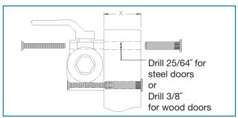
Note 1: For Thru Bolts, specify door thickness if other than 1-3/4" (44 mm). Represented in diagram as dimension "X".
