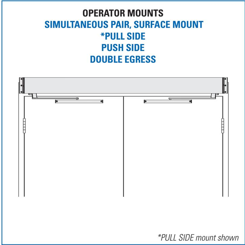
*The 9750 MIDDLE SWING® by LCN is a low-energy automatic swing door operator that is a cost-effective solution to ADA-compliance. In automatic mode, push button controls open the door automatically and permit safe, easy access for the disabled or elderly. This swing operator acts as a regular pedestrian door without automatic activation.*
