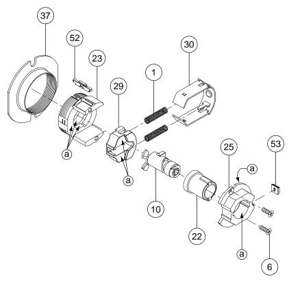
(a) Apply light film of 100% synthetic grease on surfaces with brush.
