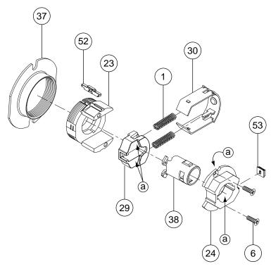
Apply light film of 100% synthetic grease on surfaces with brush.
