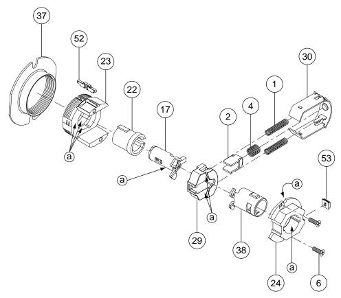
ⓐ Apply light film of 100% synthetic grease on surfaces with brush.
