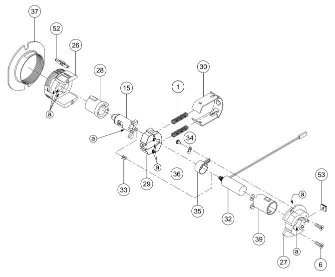
a Apply light film of 100% synthetic grease on surfaces with brush.
