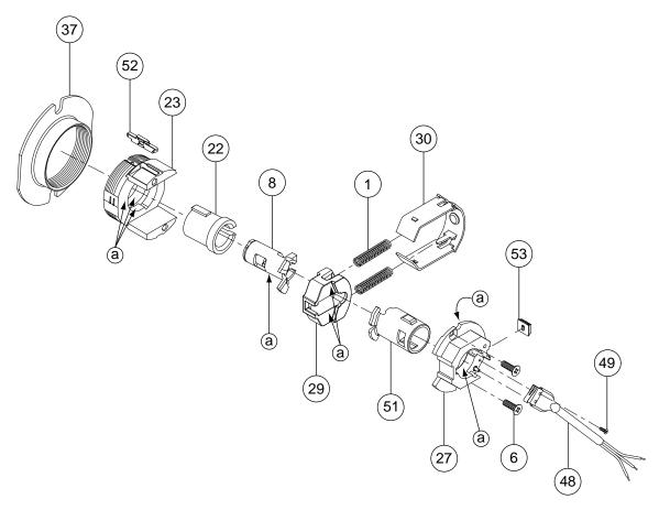
ⓐ Apply light film of 100% synthetic grease on surfaces with brush.
