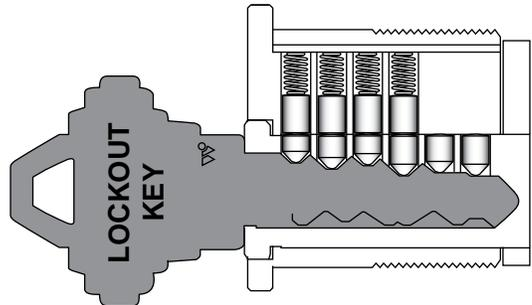
The last two notches in the key are removed allowing the key to exit the cylinder.
