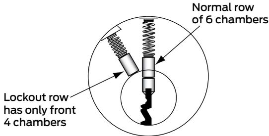
When the plug is in its standard operating position all keys will operate the lock. To temporarily disable to regular operating keys, the plug can be turned with the special key to align the bottom pins with the lockout row of pins.
