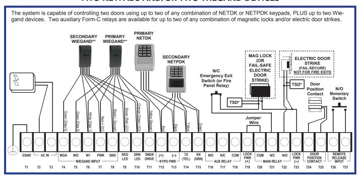
\*TSD = Transient Suppression Device (two supplied): Mount the TSD as close to the device to be protected as possible \*\*Example device shown: HID ProxPoint Plus Model 6005B.
