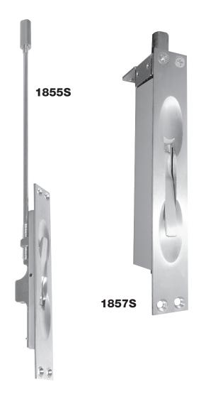
Used to lock and unlock an inactive door when the active door is open. When the inactive door is closed, moving the lock lever up locks it and moving the lever down unlocks it. Meets FED SPEC 1049: BHMA L14081: ANSI 156.16. UL Listed.
