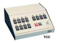
operator confusion, and simplify door supervision and control. Built-in Key lock may be used for Console On/Off or Console Lockout (UR4-8 req'd). The Key lock ensures that only authorized personnel can operate the console. The dual console interface feature allows two consoles control of a shared opening.
