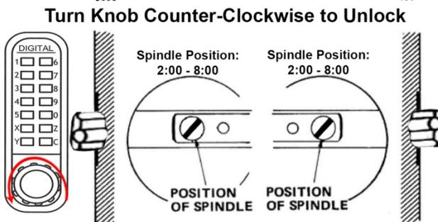
After changing the Handing Pin, the Spindle MUST be placed through the latch at a 2:00 – 8:00 angle as shown.
