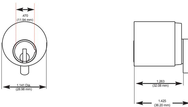
Special pinning required due to chamber height
