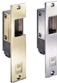
Solenoid mounts to faceplate from side with integrated spacers (1505 US4 & US26D)
