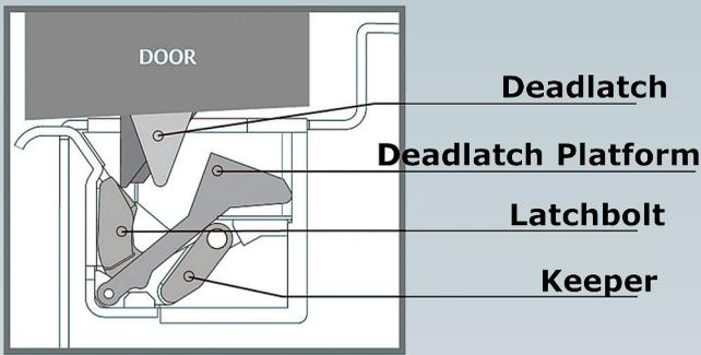
without deadbolts. It features ANSI/BHMA A156.31 Grade 1 strength with a UL10C 3-hour fire rating when used with a single door. The 8500 is ideal for use in 1-1/2" fire rated frames with a 1/2" drywall penetration, (figure 1).
